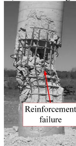
(c) Blast test [29]
