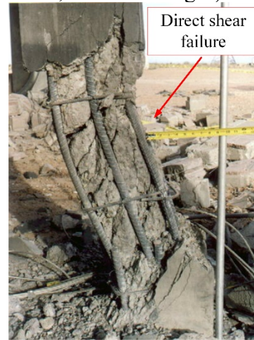
(c) Blast test [38]
